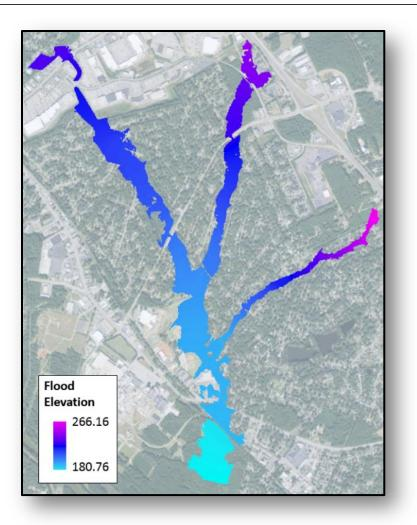
Figure 78. Water Surface Grid for Alternative A (Without Project), 100-YR Return Interval
