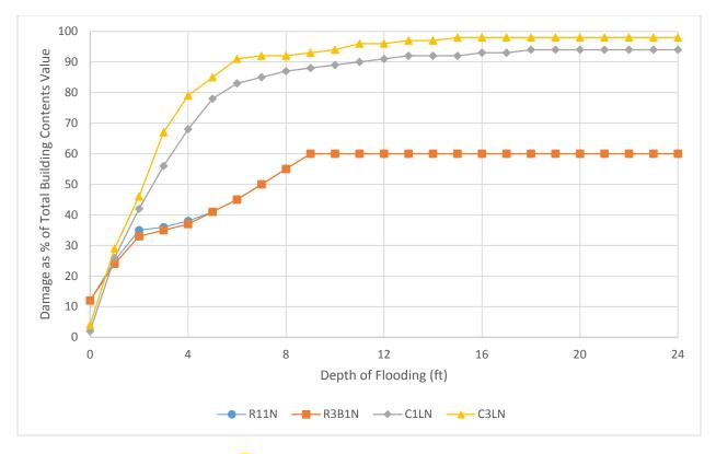
Figure **#**: Building Contents Depth-Damage Curves
