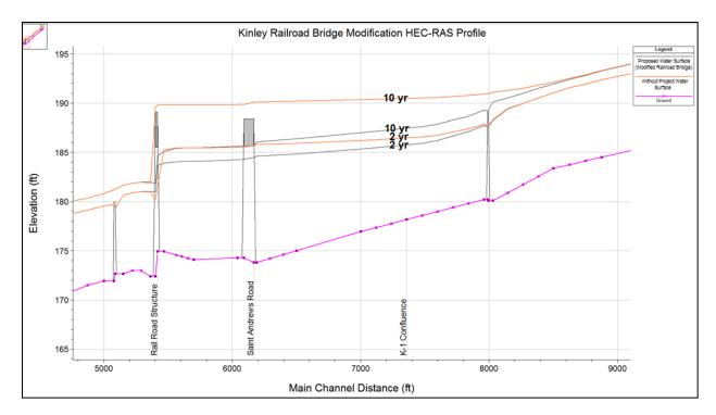
Water Surface Profiles With and Without Modifications to the Railroad Bridge
