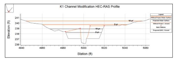
Proposed Channel Modification Cross-Section
