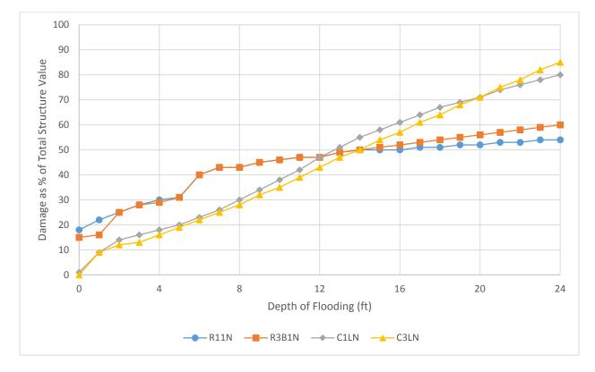
Structure Depth-Damage Curves
