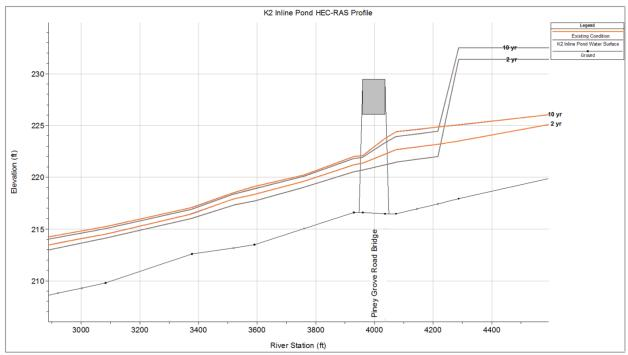
Figure #: 2-yr and 10-yr Water Surface Profile on K2 with Inline Pond
