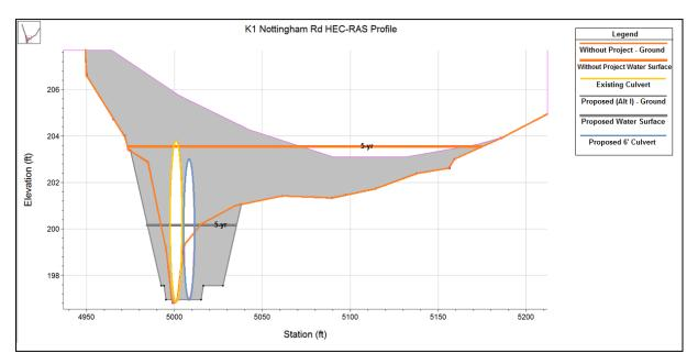
Proposed Nottingham Road Culvert Addition and Associated Reduction in Water Surface Elevation
