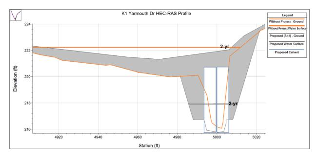
Figure X. Proposed Yarmouth Dr Culvert and Associated Reduction in Water Surface Elevation (At Inlet)
