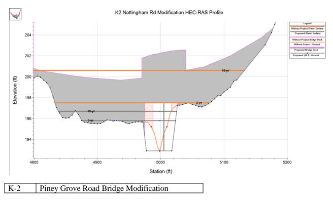
Piney Grove Road is owned by SC DOT and K-2 crosses under it through a bridge. Piney Grove Road Bridge has low-slope abutments of rip-rap that extend into the channel and rip-rap that extends upstream and downstream of the bridge. The rip-rap reduces the capacity of undersized channel. Abutments were modified in conjunction with the channel in HEC-RAS in order to provide additional capacity. Water surface elevations were lowered, as shown in Figure X.
