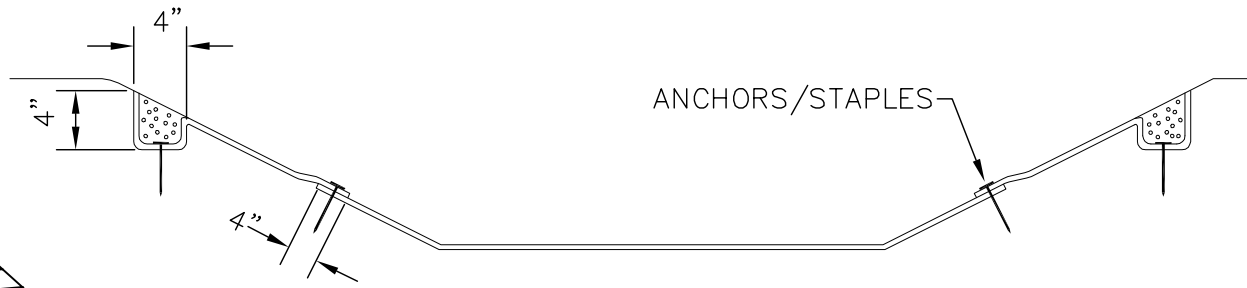
TYPICAL CHANNEL INSTALLATION
